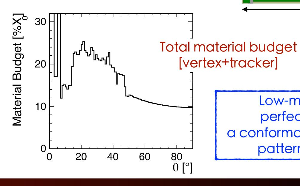
Low-mass detector perfectly suited for a conformal-mapping based pattern recognition
