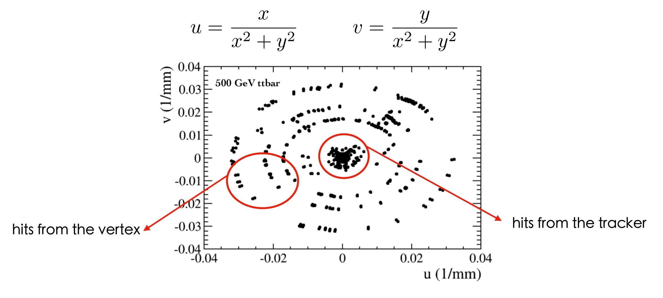
Pattern recognition in conformal space via cellular automaton, used to perform straight line search
