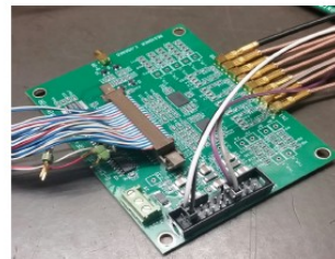
ToT board - front-end charge-to-Time-Over-Threshold conversion:
