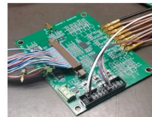
ToT board - front-end charge-to-Time-Over-Threshold conversion:
