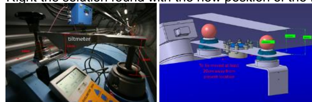
On the left, standard LHC tool for measuring roll angle. On the right, tool interfering with the DN100.
