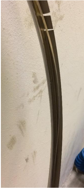
Broken Gasket from beginning of 2017
