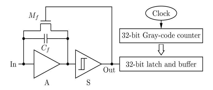
Clock: local (within ASIC) oscillator free-running at 50 – 100 MHz Basic datum is 64 bits: 32 bit time, pixel addresses, ASIC ID, ...
