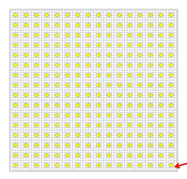
Local clock interrogation signal enters at any corner of tile, and propagates as a wave to any neighbor
