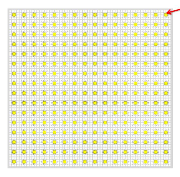
Local clock interrogation signal enters at any edge of tile, and propagates as a wave to any neighbor
