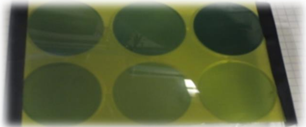
EBT3 Films irradiated with different doses
