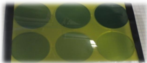
EBT3 Films irradiated with different doses
