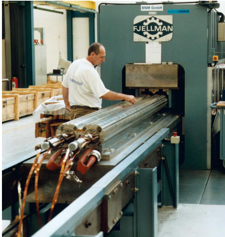
Collaring of a dipole magnet
