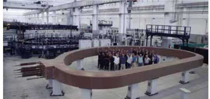
*One of ITER superconducting toroidal field coil built in Italy, ready to ship to ITER. © Let there be Light.*
