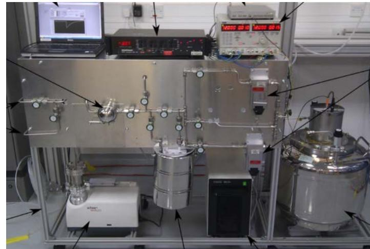
Rn concentration line for Rn measurements
