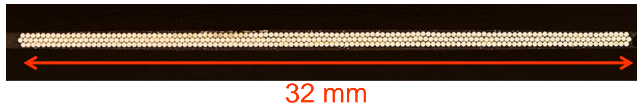
ribbon profile: 3 x ~125 fibers (prototype)
