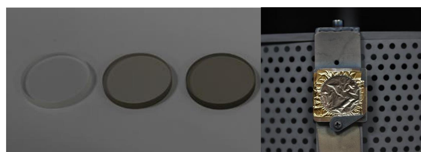
DLC for Radiation-hard photocathode 3 mm MgF 2 + DLC (different thickness)
