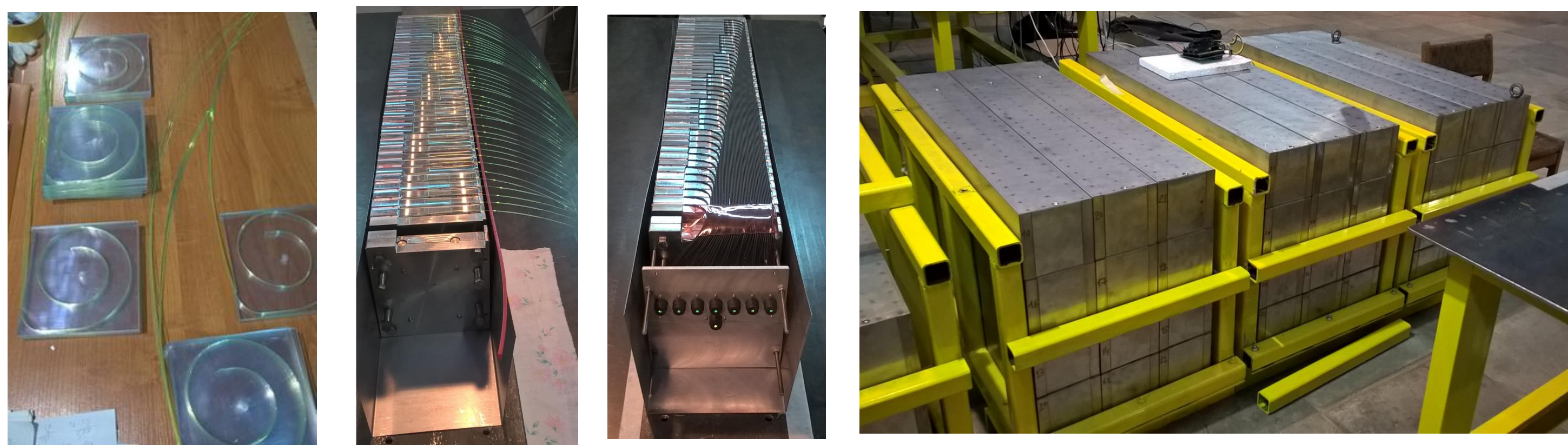
Fig.2 Photos of the different stages of FHCAL module production. Left – scintillator tiles with the glued WLS-fibers. Center – module with lead/scintillator sandwiches before and after WLS-fiber aligning. Right – assembled modules.
