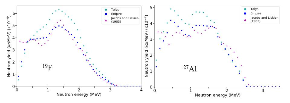
Neutron spectra from 5.5 MeV alphas in fluorine and aluminium.
