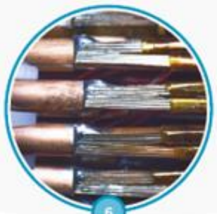
6 SUPERCONDUCTING LINKS Electrical transmission lines based on a high-temperature superconductor to carry current to the magnets from the new service galleries to the LHC tunnel.
