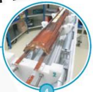
4 BENDING MAGNETS 2 pairs of shorter and more powerful dipole bending magnets to free up space for the new collimators.
