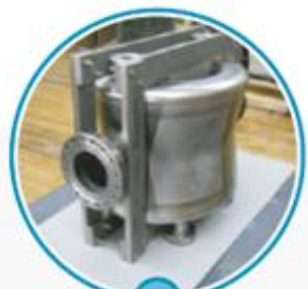
3 “CRAB” CAVITIES 8 superconducting “crab” cavities for each of the ATLAS and CMS experiments to tilt the beams before collisions.
