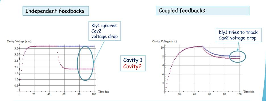
Cavity voltage following a unit step of both klystrons at time zero, and a half-unit step reduction of klystron 2 alone at time 50.
