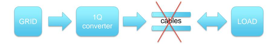
With the new SClink, a 2-quadrant converter is required to recover the magnets energy (40 MJ).
