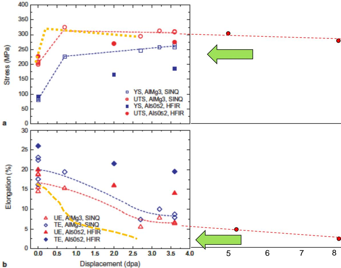
Fig. 9. The irradiation dose dependence of (a) yield stress (YS) and ultimate tensile strength (UTS), (b) uniform elongation (UE) and total elongation (TE). For a comparison, a few data of Al-5052 irradiated in the HFIR [8] were included.
