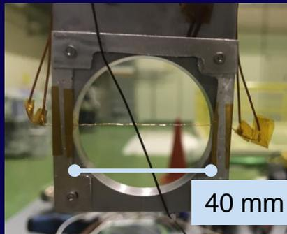
Under cryotemperature ( $\sim 20$  K), displacement cross section ( $\sigma$ ) was obtained by increase of resistivity ( $\Delta\rho_{Cu}$ ) due to proton irradiation with average flux ( $\overline{\phi(E)}$ )
