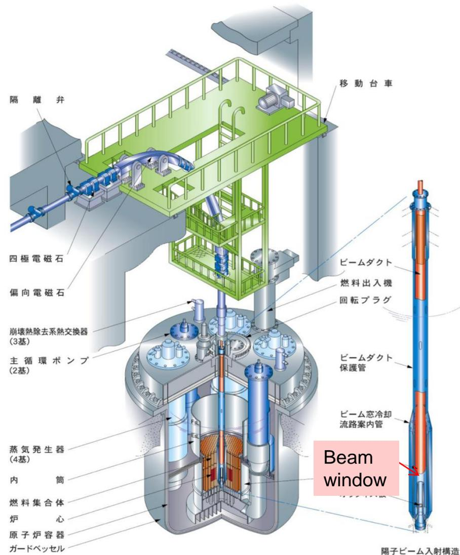
• Beam window: 20 dpa/year. Accuracy of dpa is required for damage estimation.
