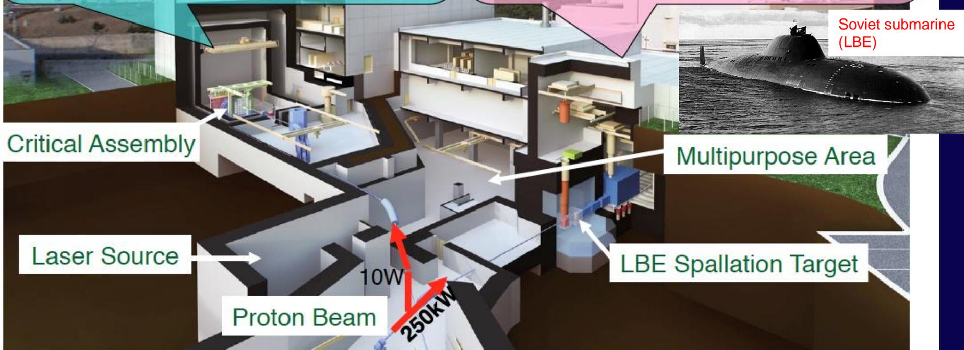
For R&D of ADS, 0.4 GeV beam by LINAC will be delivered to TEF.
