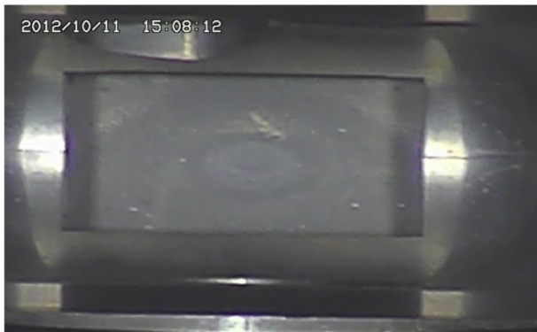
JSNS Beam Window inspected after ~1000 MW h of operation
