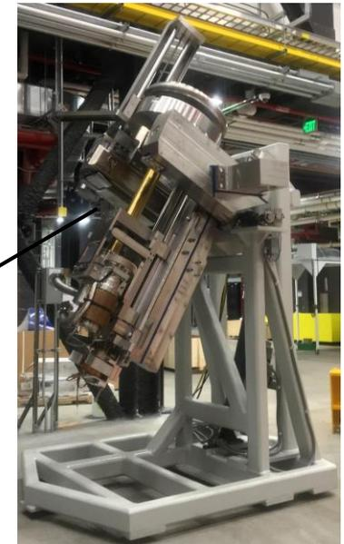
Beam dump module mounted on integration frame
