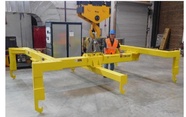
Vessel seal retainer lifter
