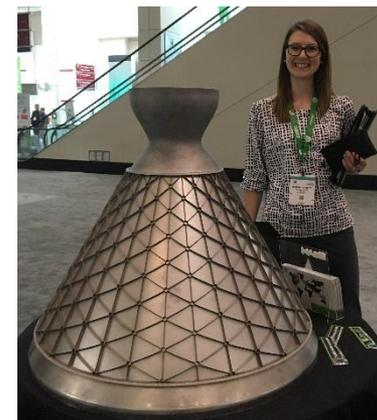
3D printed object with similar size than FRIB beam dump
