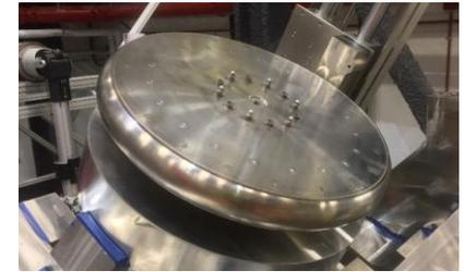
Titanium beam dump drum with 1-mm shell
