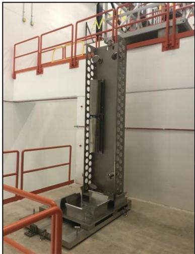
Thermal Imaging System mounted on the target vessel mounting frame
