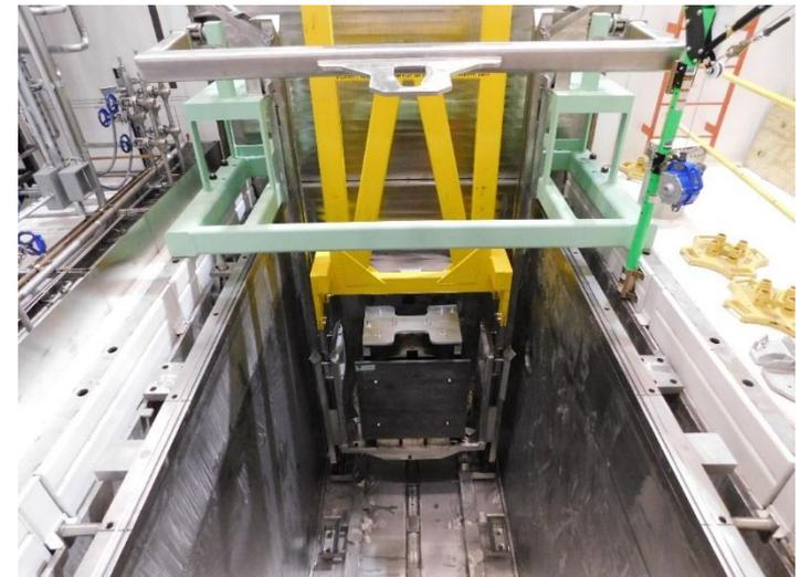
FSQ5-magnet yoke in cradle placed in WIQ4 position using complete set of remote handling tooling
