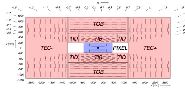
Silicon Tracker: PIXEL (blue) refers to silicon pixel detectors while TIB, TID, TOB and TEC (red) all refer to silicon strip detectors
