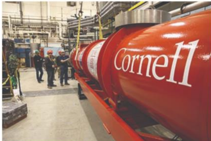
The main linac cryomodule
