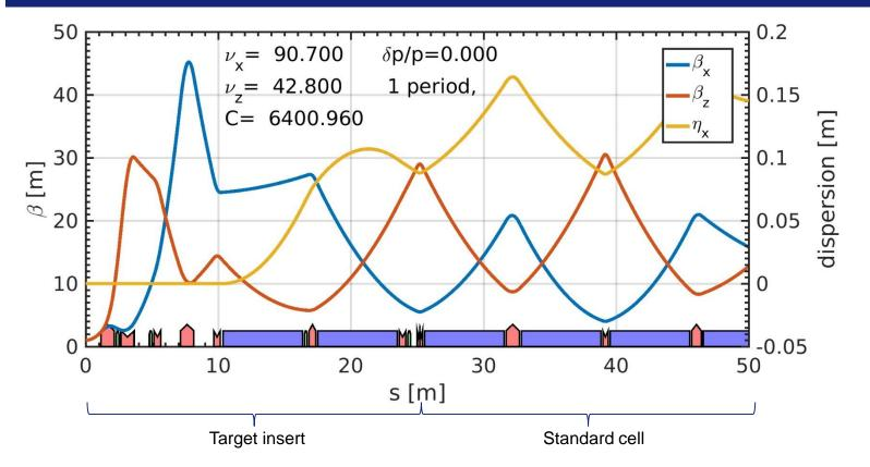
Target optics designed only to study target interaction with given optics functions. The target interaction region optics, including dipoles for positron-muon beam separation and adequate chromaticity correction, need to be designed.
