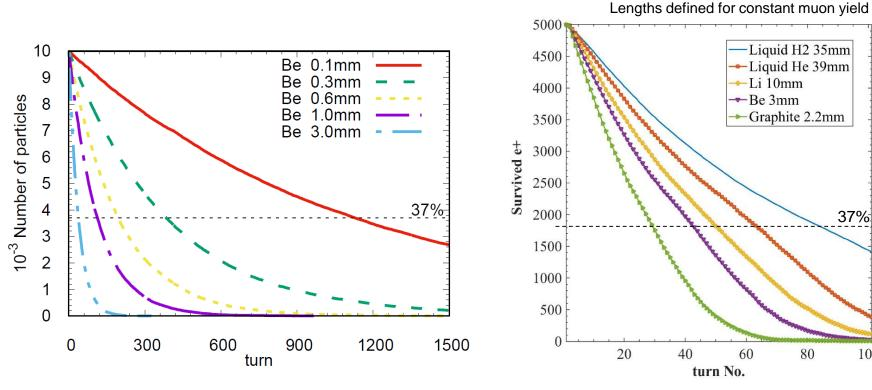
Improved Lifetime for LH2, LHe and Li but larger thickness increase multiple scattering and thus the intrinsic muon emittance
