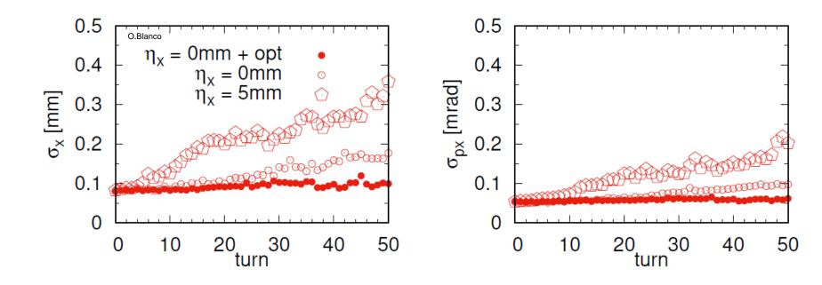
Tracking simulations confirm that the small beta functions and zero dispersion at the IP cancel the degradation of the positron beam size due to the interaction with the target.
