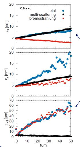
Positron beam interaction with 3mm Be target: separated contributions of multiple scattering and bremsstrahlung.
