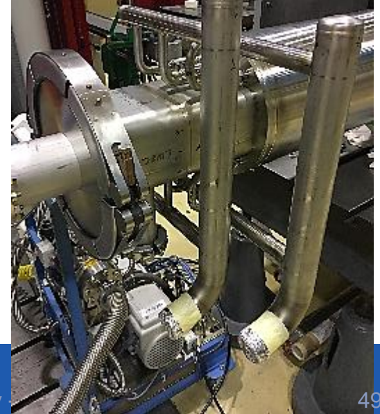
Final leak detection (upstream w/ water manifolds)
