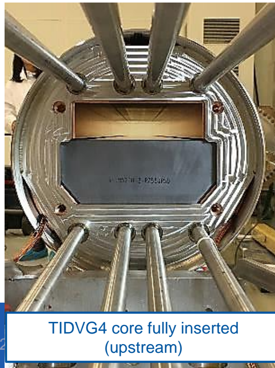
TIDVG4 core being pulled into the vacuum chamber
