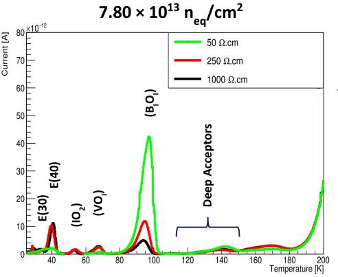
There is a clear dependence of the B<sub>i</sub>O<sub>i</sub> peak with the initial Boron concentration. Suggesting that the main mechanism for acceptor removal is:
