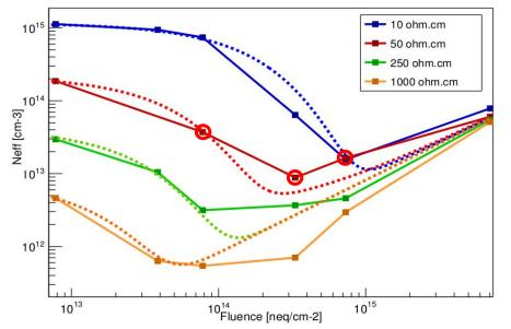
The shape of the TCT waveform could not be used to check sign inversion because the sensors are just 50  $\mu$ m. But by comparing the charge collected over bias for different light injections, **it was possible to verify type inversion**.
