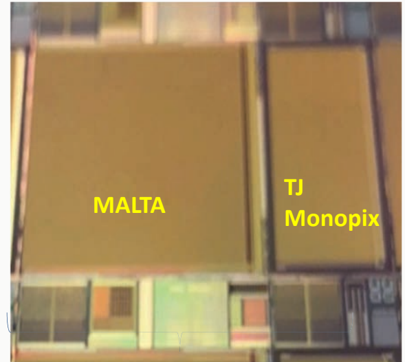
MALTA TJ Monopix TowerJazz 180 nm epitaxial (25 \mu\text{m} ) substrate \rho > \text{k}\Omega \text{ cm}
