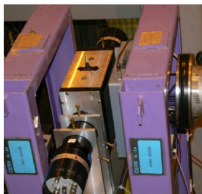
Z 2 detector, Be run (Cherenkov in Quartz)
