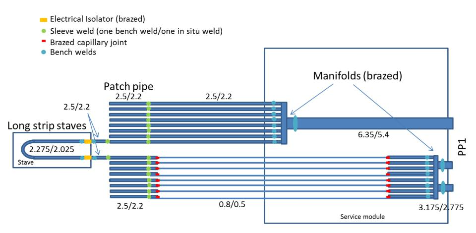
Tube dimensions are OD/ID for illustration only – final numbers slightly different Units of measurement in mm
