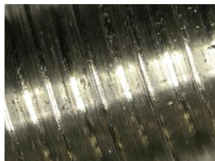
2024-T4 No Coating, after No galling, turning nuts still easy
