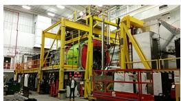
**GlueX Experiment** (Jefferson Lab, Hall D): characterization of 2800 Multi Pixel Photo Counters (MPPC), manufacture of 4000 lightguides *etc.*
