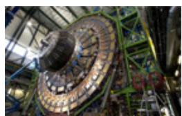
**ATLAS Experiment** (CERN): manufacture part of small-strip Thin Gap Chambers (sTGC) for the Muon Small Wheel (140 detectors)
