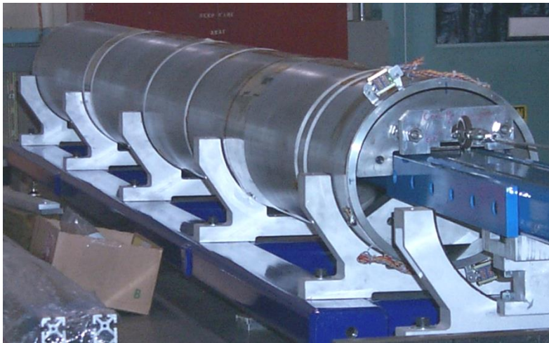
Structure re-assembly with segmented shell
