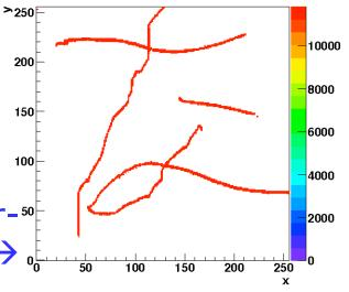
Locally induced noise, "written" to Timepix surface with a pulser and an insulated wire  $\rightarrow$
