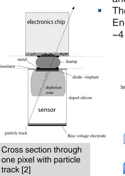
and digitalized by Timepix (depending on the sensor either electrons or holes). The duration of the pulse is measured per pixel in energy mode. Energy range per pixel after calibration with known sources of ionising radiation: ~4 keV up to several MeV
