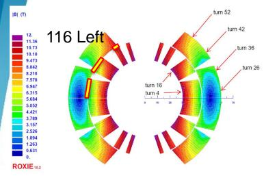
Cycle 5 1.9 K 12 W/m in 1 quadrant coil 116 12.27 kA
