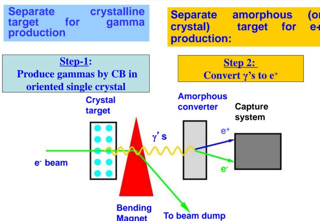
**Target#1:** uses an aligned single crystal diamond as a radiator for an electron beam to make a photon source instead of using an amorphous target. We will exploit the enhancement of photon radiation via the mechanism of **Coherent Bremsstrahlung (CB)**[3]. Additionally, if the incoming electron beam is longitudinally polarized, then the produced photons are circularly polarized due to conservation of angular momentum [4].
