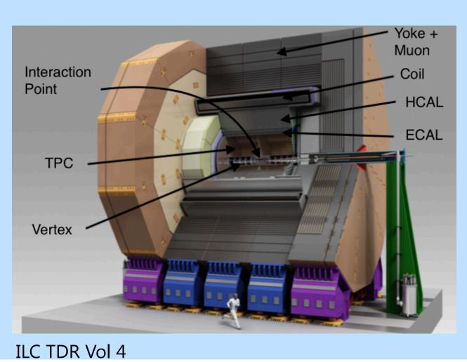
◄ The detector used for this analysis is the International Large Detector. The detector has a very similar design to Compact Muon Solenoid detector at the LHC. Similar performance is expected for the CLiC-like Detector.
