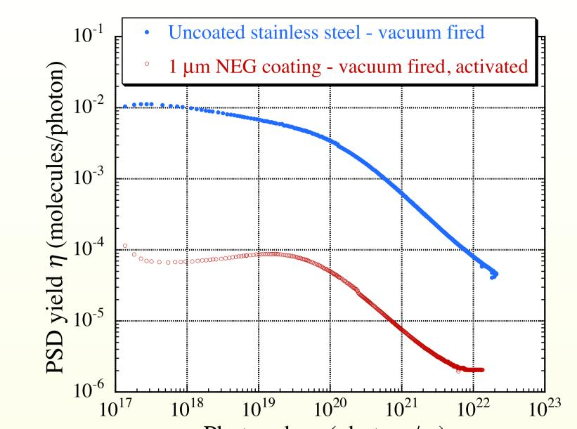
PSD yields quickly reach **10-<sup>6</sup> molecules/photon**, the same order as those of standard 1-μm NEG coatings and about two orders of magnitude lower than uncoated surfaces.
