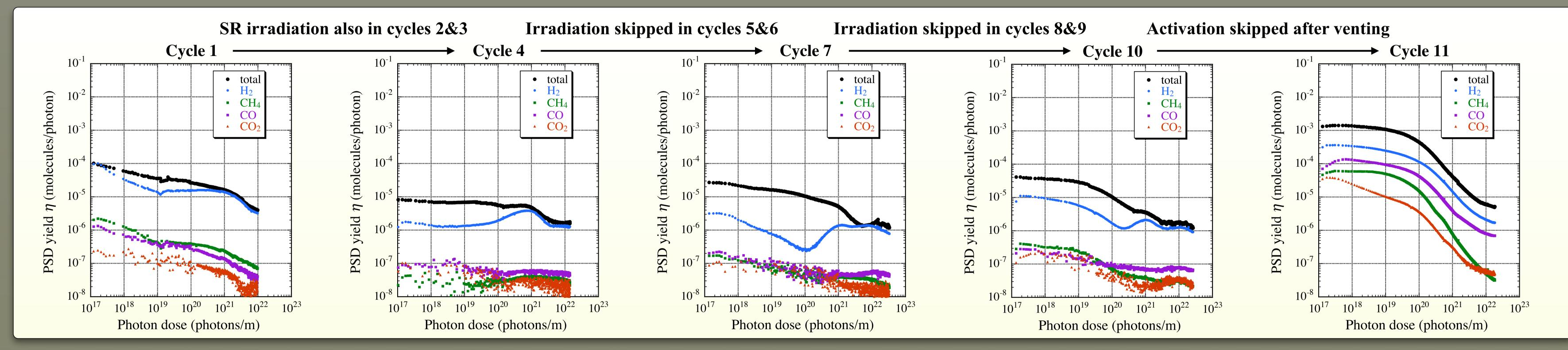
Composition ratio in the PSD outgassing was similar to those of standard 1 μm thick NEG coatings. CH4 desorption was low enough for application to a real machine.
