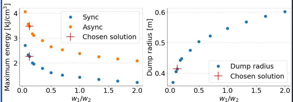
Chosen solution at  $w_1/w_2 = 0.125$ : safely below damage threshold, and has a small dump size. Easy tuning in the “energy-dumpsize” trade-off.
