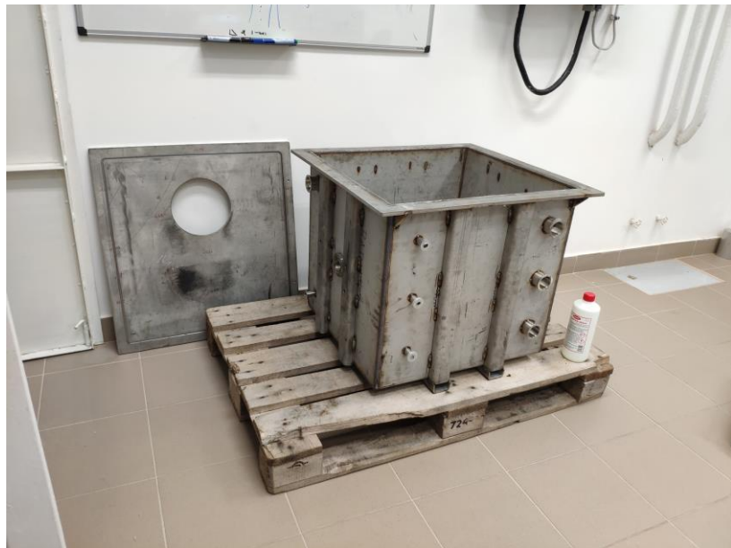
Vacuum epoxy impregnation system, winding machine being prepared
