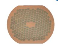
15% Rolling used to simulate the wire deformation during cabling
