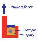
Wire impregnated with epoxy applied stress uniformly distributed
