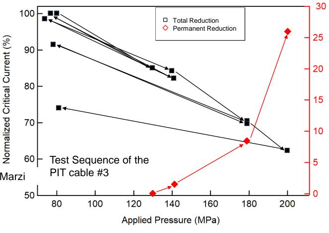
Onset permeant reduction ~130 MPa, up to ~ 180 MPa most likely due to plasticization of copper afterwards, to cracks in the filaments
