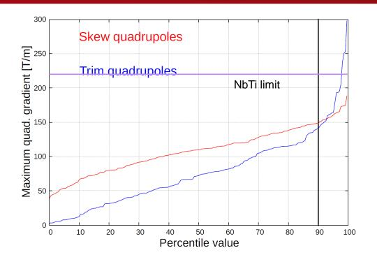
Orbit corrector strengths compatible with NbTi technology at 90% level
