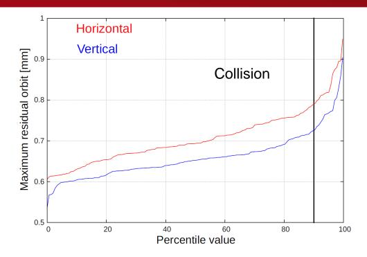
Residual orbit < 1 mm at any point of the synchrotron, in accordance with the geometry of the dipole chamber (5 mm aperture)
