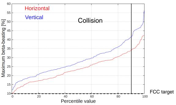
Beta-beating too strong, well above the 10% target in most machines at injection, in all machines at collision
