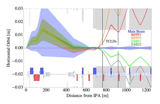
**Dispersion Suppressor Collimator (TCLDs)** positions for p-p can also **absorb secondary beams** from Pb-Pb collisions.
