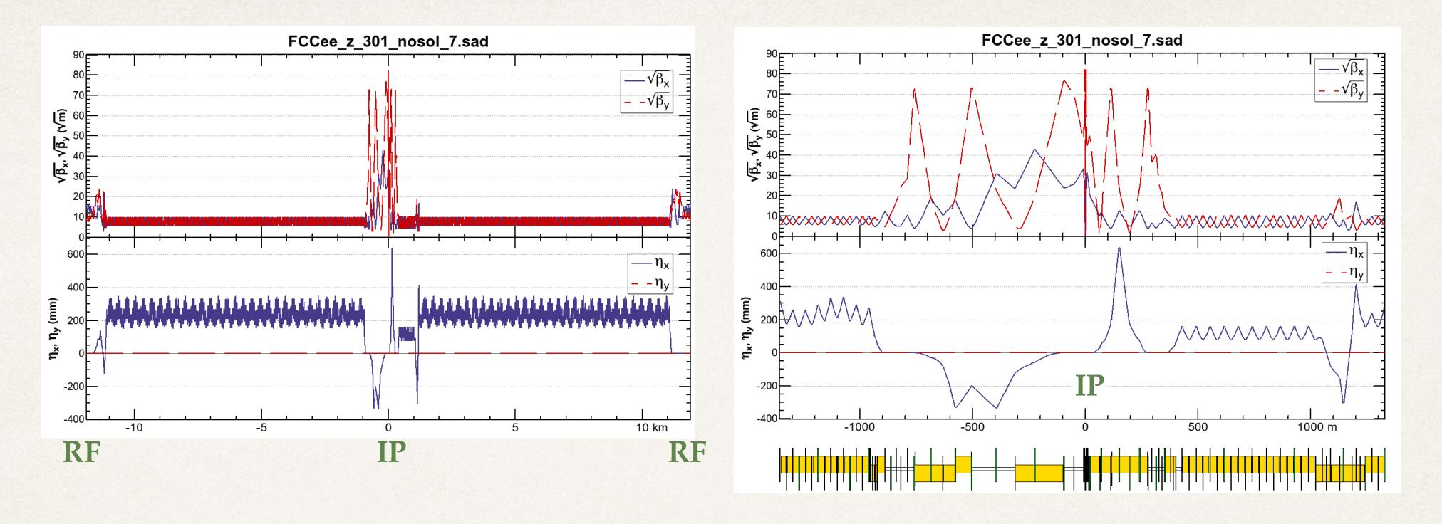
\*  $\beta_x$ \* is reduced to 10 cm (CDR: 15 cm) to suppress the x-z coherent instability (D. Shatilov).
