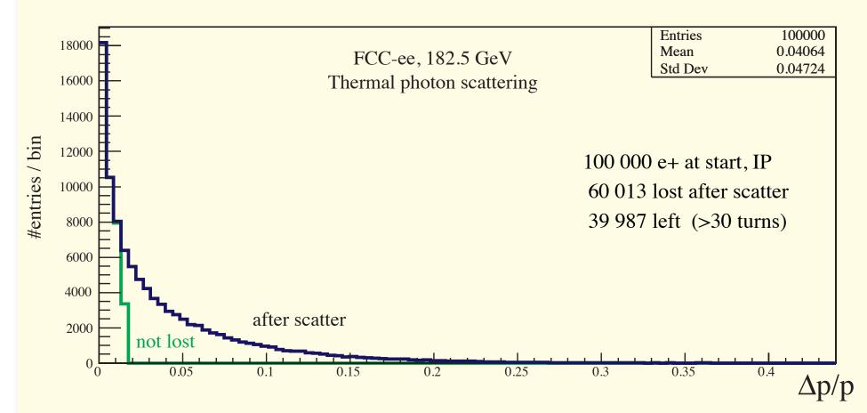
At present : using the ideal lattice translated from SAD. Solenoid, apertures, beam2 added by hand granularity by element boundary : generation, aperture checks at end of elements no errors, no misalignment, gaussian beams, RF and radiation here turned off energy acceptance bit smaller and detuning with amplitude a bit larger than with SAD
