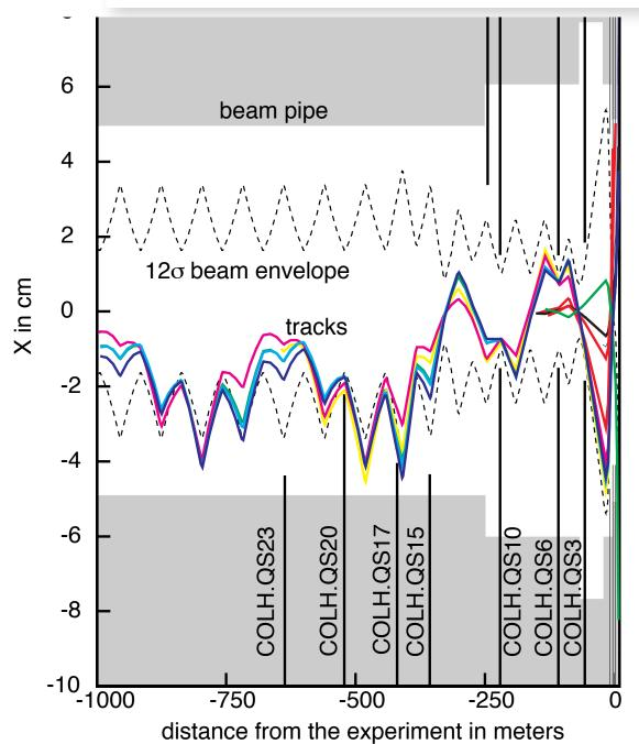
Illustration of beam particle tracking through the LEP lattice over 1000 meters up to an experimental region (cs coordinates). The distance X from the nominal orbit is given in cm units.
