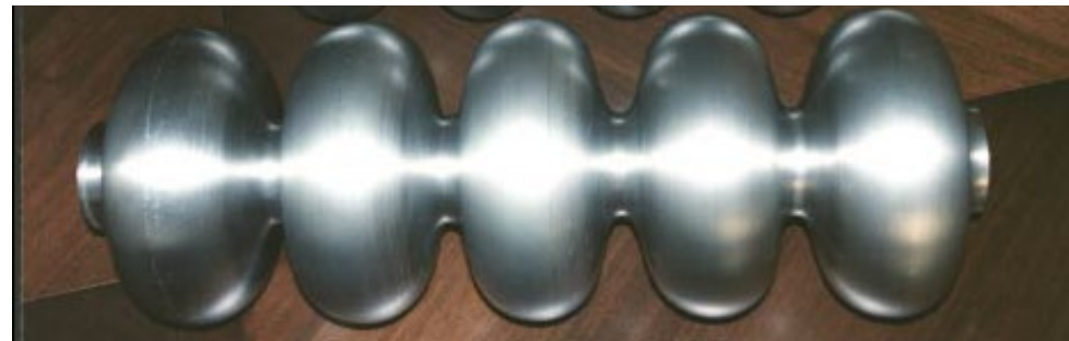
First seamless multicell by spinning
