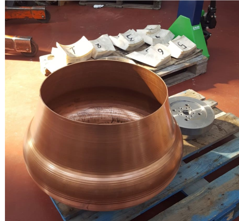
READY FOR THE SPINNING OF 2° HALF CELL
