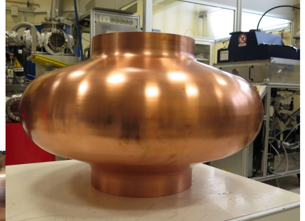
Spinning of Cavity #2 completed
