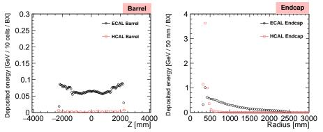
Energy deposits reach up to 0.1 GeV / 10 cells in ECAL Barrel and 4 GeV / 50 mm in HCAL Endcap
