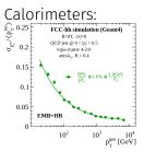
Jet energy resolution of the barrel calorimeters standalone
