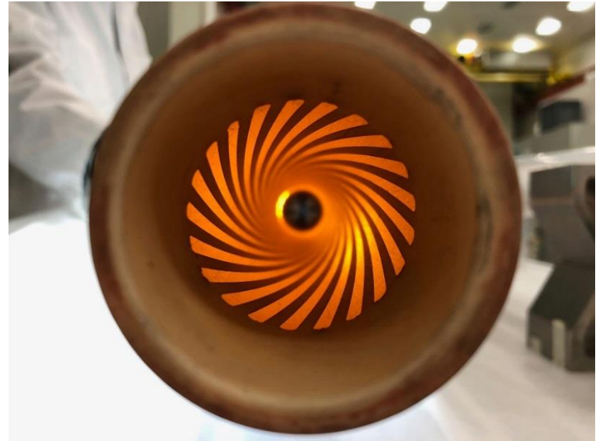
Prototype alumina tube with spiral screen conductors
