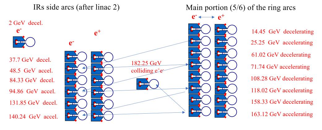
Small gap magnets with 5 mm gap Prototyped for eRHIC at 0.43 T: FCC ee needs only 0.04 T, e.g. it is very low power consumption magnet
