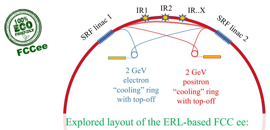
Flat electron and positron beams are cooled in 2 GeV cooling rings with top-off injection to keep intensity constant
