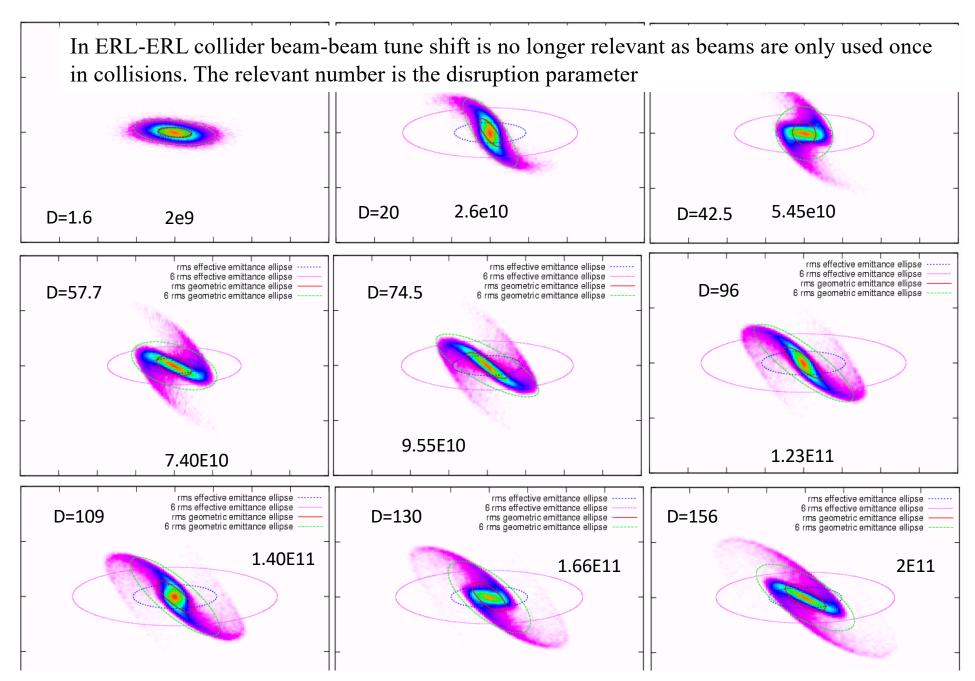
As part of the ERL-based eRHIC studies it was demonstrated that disruption parameter up to 200 for electron beam colliding with hadron beam can be tolerated: transverse beam emittance will double in a single collision, but the beam than can be comfortably energy recovered. Important note: this assumption has to be confirmed by direct simulation of colliding electron and position beams.
