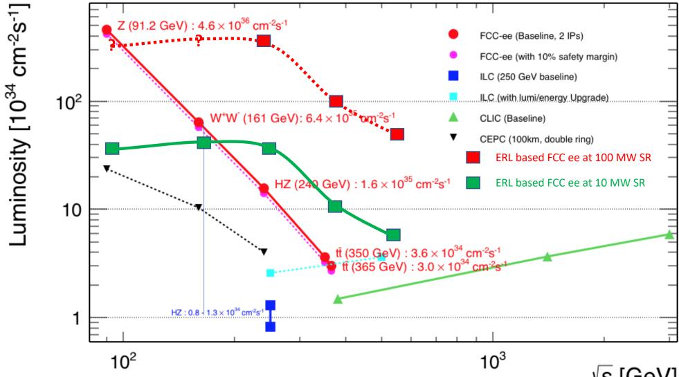
Luminosity can be shared (split) by multiple detectors by alternating beam collision points. **VS [GeV**]
