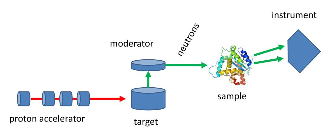
"spallation" is the process that releases neutrons from the target nuclei
